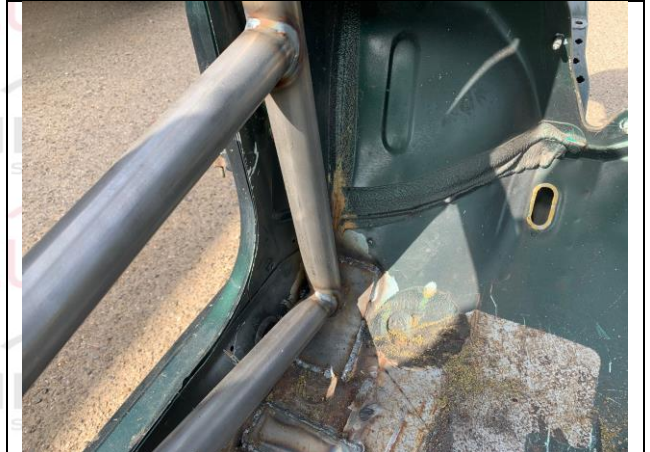
PHOTO 4 MAIN ROLLBAR TO FLOOR ATTACHMENT
