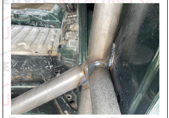
PHOTO 8 MAIN ROLLBAR TO "B" PILLAR ATTACHMENT
