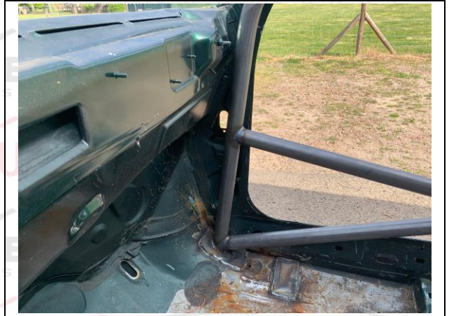
PHOTO 6 FRONT ROLLBAR TO FLOOR ATTACHMENT
